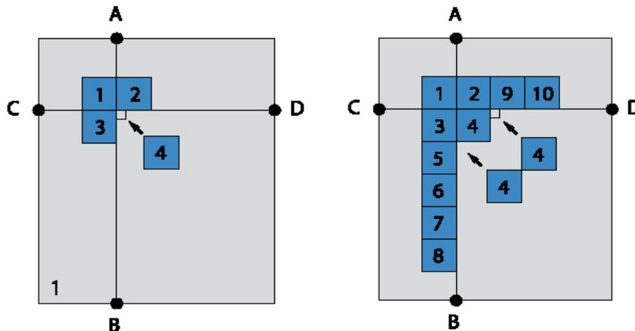
When laying on raised floor subfloor, the tiles are aligned in a form identical to the raised floor plates (generally 60 x 60 cm) as per the existing raised floor pattern. The centre axes of tiles are aligned on the joints of the raised floor plates. Thus, a tile generally rests on each of the four raised floor plates.
